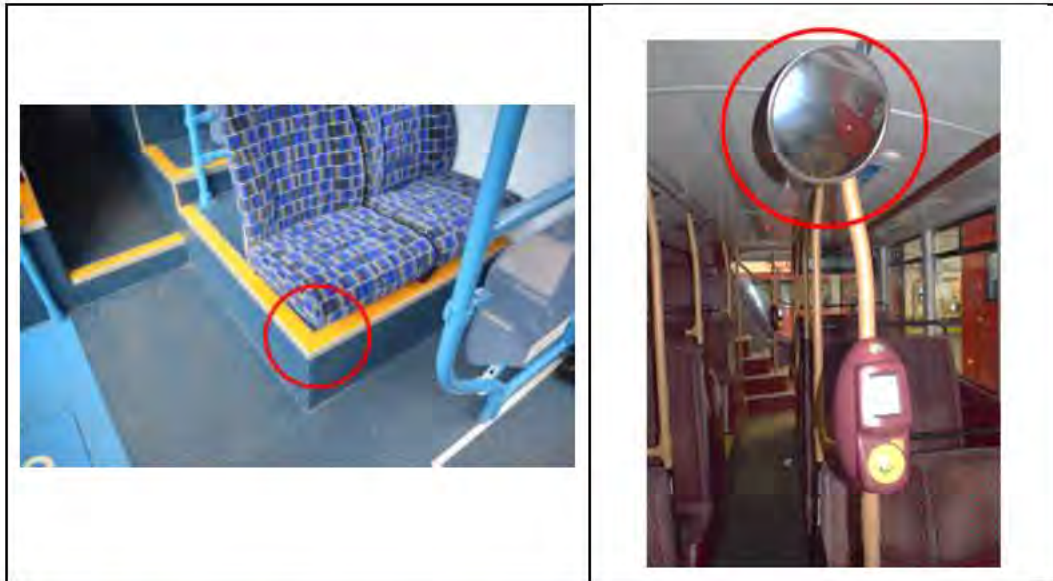
Figure 34_7: Examples of general hazards for standing passengers, corner of step (left) and mirror in head impact zone (right).
