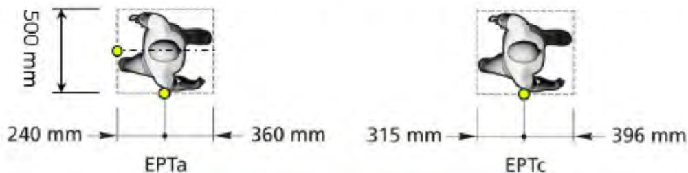
Figure 15_4: Virtual box around EPT
