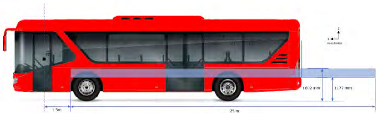
Figure 19_14: Side view of wide-angle assessment zone
