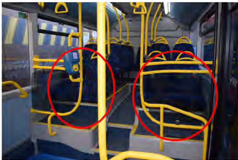
Figure 34_1: Examples of seats with high occupancy rate immediately adjacent to a door and only accessible via a step.
